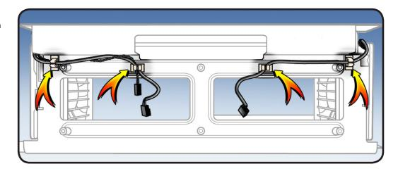
**27** Release **4** latches on front fan and slide fan out of cage.
